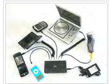
Auxiliary charger designed to fit a variety of proprietary devices
