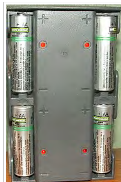
This unit charges the batteries until they reach a specific voltage and then it trickle charges the batteries until it is disconnected.
