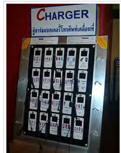
Pay-per-charge kiosk, illustrating the variety of mobile phone charger connectors
