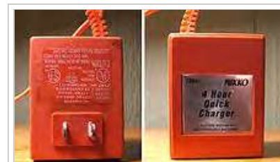
A simple charger equivalent to an AC/DC wall adapter. It applies 300mA to the battery at all times, which will damage the battery if left connected too long.
