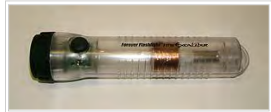
Linear induction flashlight, charged by shaking along its long axis, causing magnet ( visible at right ) to slide through a coil of wire ( center ) to generate electricity
