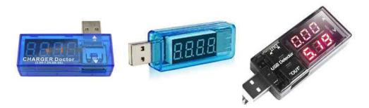
The USB mah meter can also be used to measure voltage and current. You might find it usefully if you charge anything using a USB source. The item would be charged when current flow goes to zero. This meter then indicating how much charge the item took in units of mah. This mah is the number of ma or one thousandth of an amp the battery will supply for one hour.
