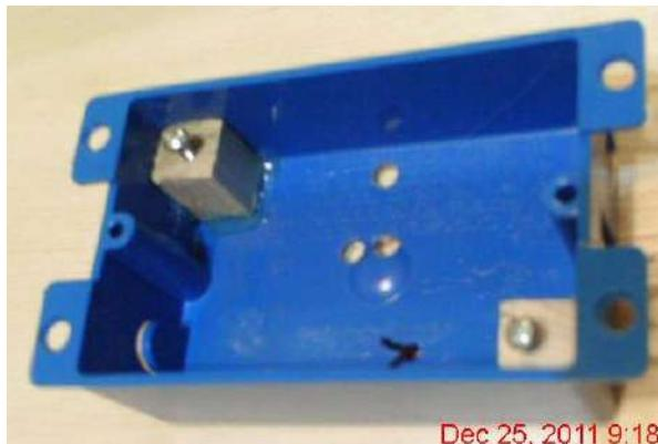
For buzzer circuit the stand off minimum height of .75" for one 3/8" wooden square dowel and one 1/2" wooden square dowel. For all the rest used two .75" long by 1/2" x 1/2" wooden square dowel. Two #4 by 1/2" round head sheet metal screws are used to hold down the PC board. See above for how this looks once it is glued in with hot melt glue.
