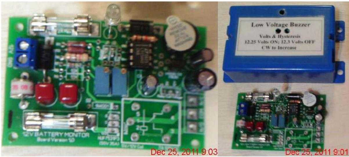
The above is how the low voltage Buzzer circuit ends up looking. Note that it doesn't need to have any of the output relay circuit components filled in.
