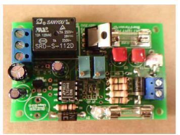
A Dump Load Controller is next shown: Note the extra two 10 Mohm resistors.
