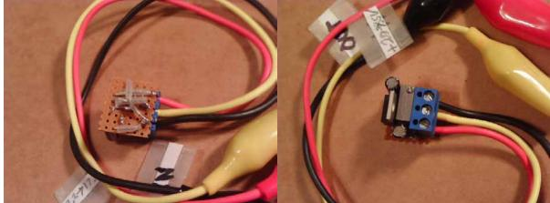
A small piece of project PC board was used. Note the adjustment 25 Turn pot in the center. **Labels for boxes:**
