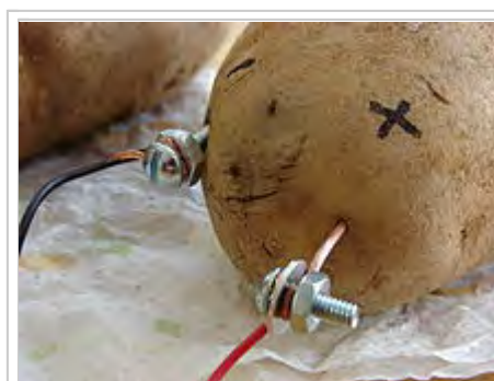
Potato battery with zinc (left) and copper electrodes. The zinc electrode is a galvanized machine screw. The copper electrode is a wire. Note the labels – and + marked on the potato indicating that the copper electrode is the positive terminal of the battery. A short screw and nut connect the electrodes to the copper wires that have black and red insulating plastic coatings.
