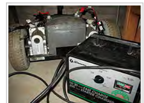
Charge current needs to match the ability of the battery to absorb the energy. Using too large a charge current on a small battery can lead to boiling and venting of the electrolyte. In this image a VRLA battery case has ballooned due to the high gas pressure developed during overcharge.
