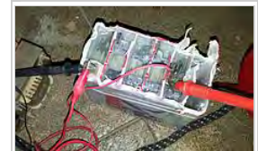
An opened two-wheeler self-starter battery
