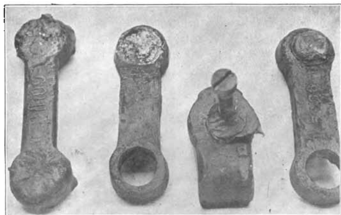
Fig. 186. Trouble Breeders. Failures in Making Connections and Burning In
