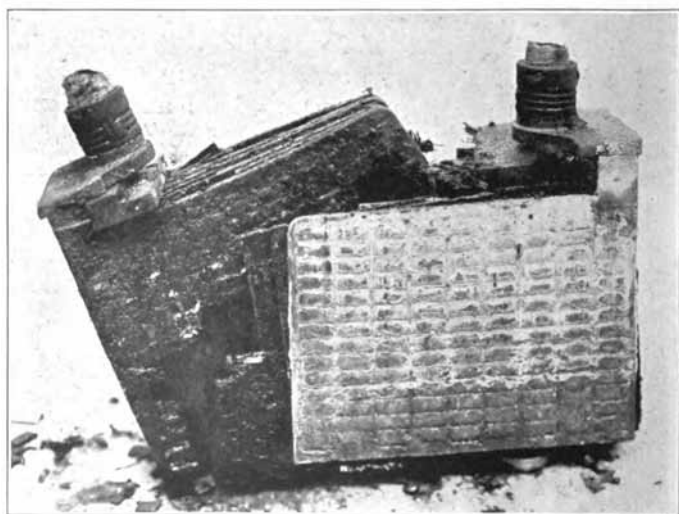
Fig. 120. Corroded, Bulged and Sulphated Negatives. Disintegrated, Rotted Positives
