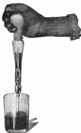
Fig. 24. Release the Pressure on the Bulb, Thus Drawing Water Up into the Hydrometer
