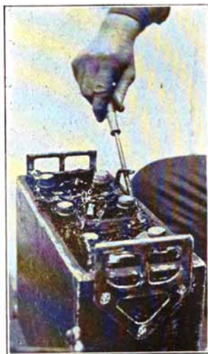
Fig. 109. Removing Compound from Edge of Case and Tops of Jars with Hot Screw Driver
