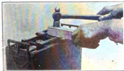
Fig. 129. Tapping Connectors in Place, Preparatory to Charging after Battery has been Opened and Shorts Removed
