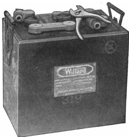
Fig. 18. Battery Short Circuited by a Pair of Pliers
