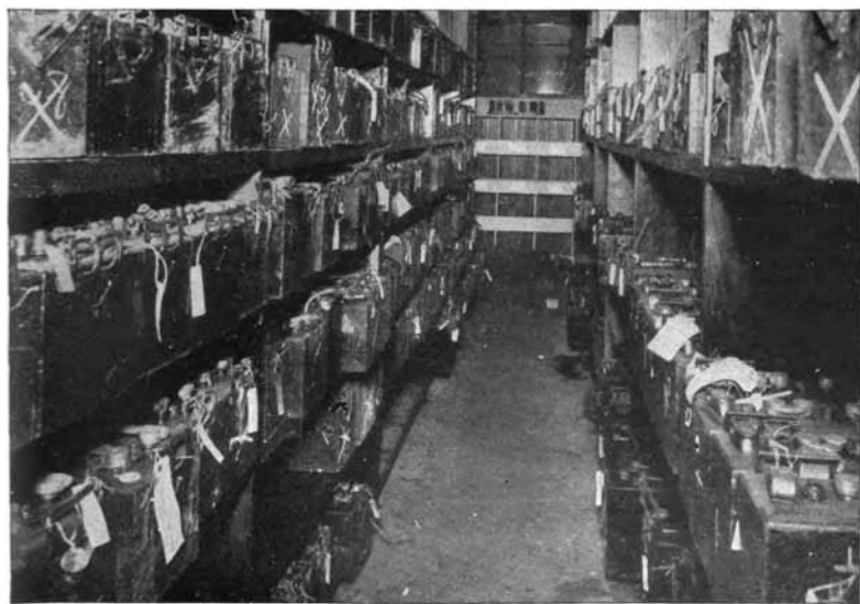
Fig. 57. Typical Stockroom Showing Heavy Shelving Necessary for Storing Batteries
