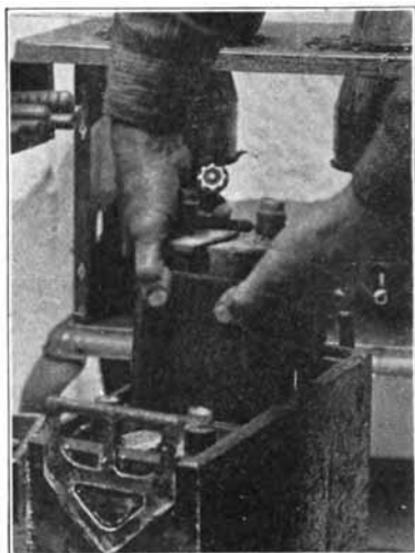
Fig. 142. Tightening an Element in Jar by Placing a Separator on Outside Negative
