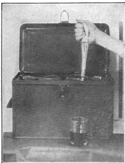
Fig. 25. Insert the Tube in Vent Hole in Center of Battery, and Squeeze the Hydrometer Bulb Until the Cell is Filled to the Proper Level
