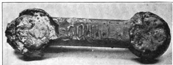
Fig. 184. Upper Side of a Very Poorly Burned-In Connector
