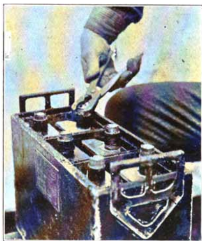
Fig. 128. Cleaning Scale From Posts Before Replacing Connectors Temporarily for Charging
