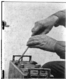
Fig. 105. Cleaning out Cracks with Screw Driver
