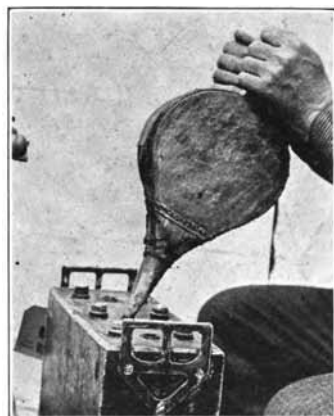
Fig. 102. Blowing Gas out of Battery with Hand Bellows
