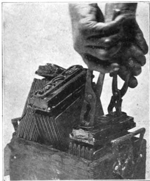
Fig. 165. Lifting Elements Out of Jars, and Resting on Edge of Case to Drain. Willard Type S Battery.
