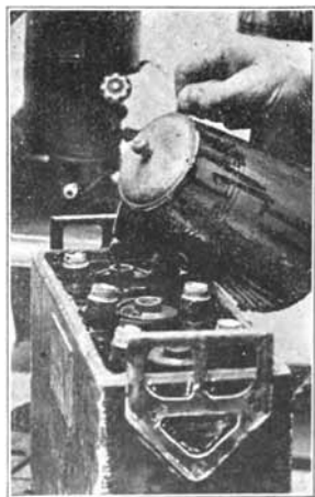
Fig. 144. Pouring Compound on Top of Lower Covers
