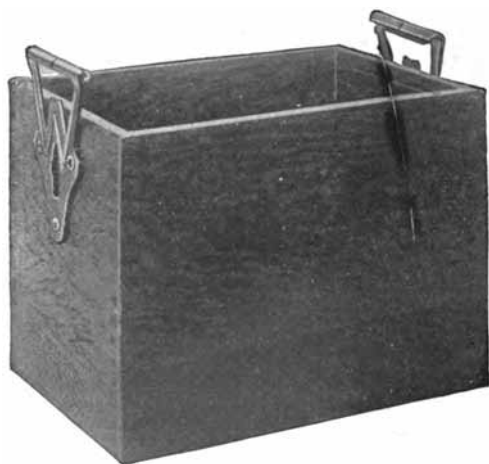
Fig. 49. Battery Box or Case with Handles. It Is Made from Kiln-Dried Oak Lumber and Thickly Coated with Acid-Proof Paint. All Metal Parts, Other Than Lead, Are Lead-Coated to Keep Them from Corrosion by the Acid in the Battery Solution.
