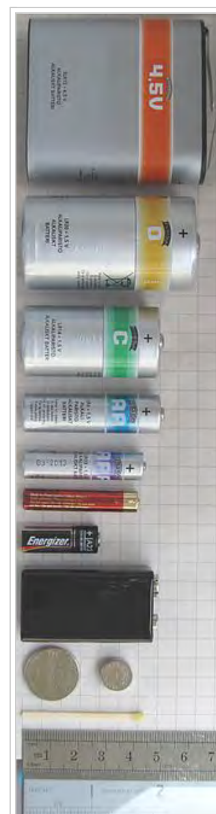
From top to bottom: a large 4.5-volt (3R12) battery, a D Cell , a C cell , an AA cell , an AAA cell , an A23 battery , a 9-volt PP3 battery , and a pair of button cells (CR2032 and LR44)
