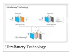
When UltraBattery and standard VRLA (used in a partial SoC regime) are compared in experimental conditions, UltraBattery has been shown to achieve about 13 times the capacity turnover of a standard absorbed glass matt VRLA battery.<sup>[1]</sup>
