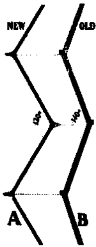
Drawing illustrating the difference between the new foundation A, and the old B. The latter has a thicker base, a flatter angle, and an unavoidable distortion. The bees greatly prefer A.
