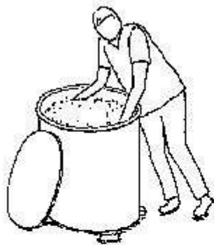
Take the intermediate trays with the used absorbent out of the chamber.
