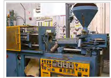
Small injection moulder showing hopper, nozzle and die area
