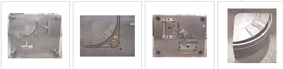
"A" side of die for 25% glass-filled acetal with 2 side pulls.
