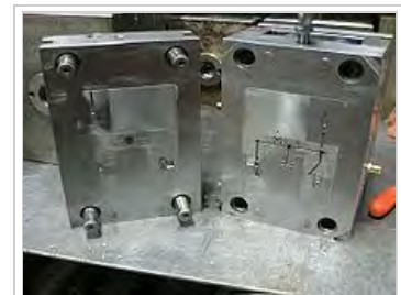
Standard two plates tooling – core and cavity are inserts in a mould base – "family mould" of five different parts
