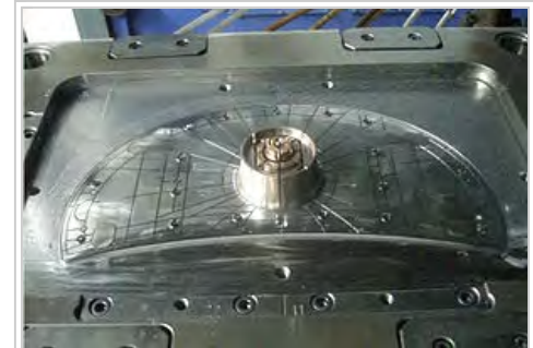
Beryllium-copper insert (yellow) on injection moulding mould for ABS resin
