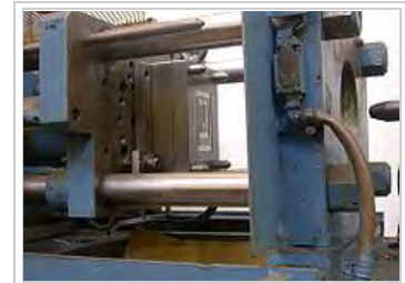
Paper clip mould opened in moulding machine; the nozzle is visible at right
