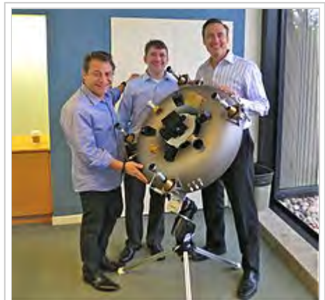
Unveiling the titanium integral space bus satellite by Planetary Resources in February 2014. The sacrificial mold for the investment casting was 3D-printed with integral cable routing and toroidal propellant tank. From left: Peter Diamandis, Chris Lewicki, and Steve Jurvetson.
