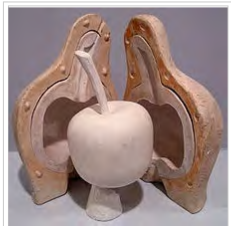
From the model a rubber mould is made. (The mould is shown here with a solid cast in plaster)
