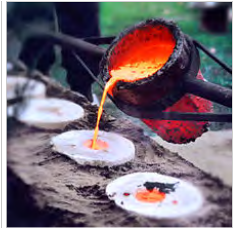
Liquid bronze at 1200 °C is poured into the dried and empty casting mould
