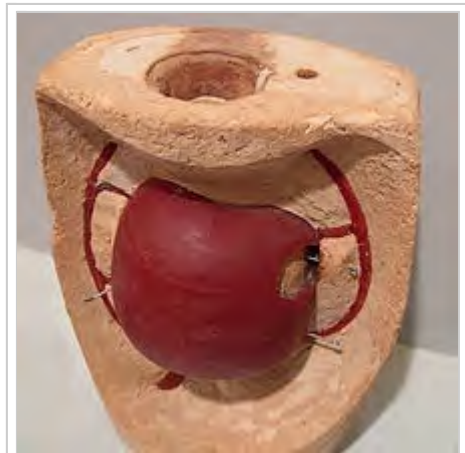
The hollow paraffin apple is covered with a final, fire-proof mould, in this case clay-based, an open view. The core is also filled with fire-proof material. Note the stainless steel core supports. In the next step (not shown), the mould is heated in an oven upside-down and the wax is "lost"
