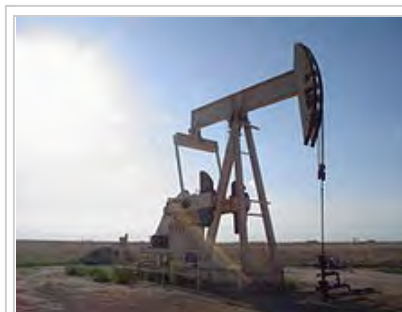
Pumpjack pumping an oil well near Lubbock, Texas
