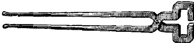
FIG. 102.—TONGS FOR HOLDING PIECES OF DIFFERENT SIZES.
