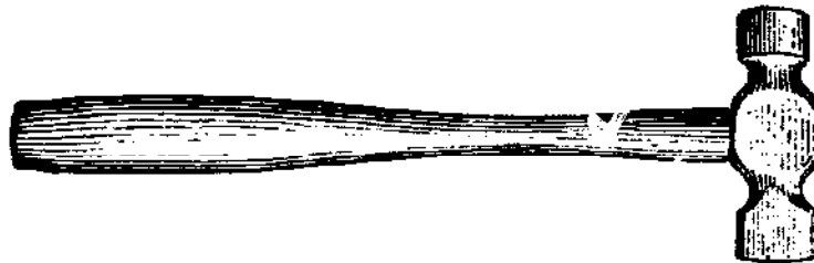
Fig. 345—Hammer Used by "J. W." in Welding Plow Points.
