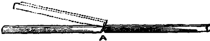
Making a Grubbing Hoe by the Method of Eph. Shaw. Fig. 365—Showing the Iron Cut for Bending Open.
