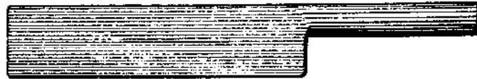
Making a Log-Chain Swivel. Fig. 275—Showing how the Piece is Flattened and Drawn Out.
