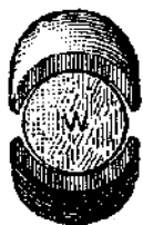
FIG. 142.—SHAPE OF TONG JAWS FOR ROUND WORK.
