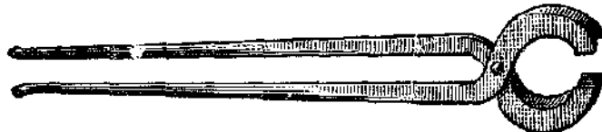
FIG. 101.—TONGS FOR BENDING IRON FLATWISE.
