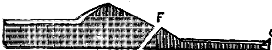
Fig. 369—Showing how the Two Pieces are Welded.
