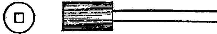
Fig. 250—Making a Valve Yoke by the Method of "Novis Homo." Side and End Views of the Stem after Drawing.
