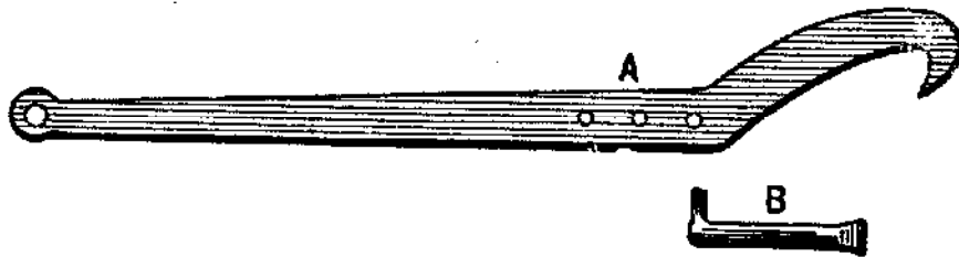
A Tool for Holding Plow Bolts. Fig. 35 – Showing how the two Pieces are made.
