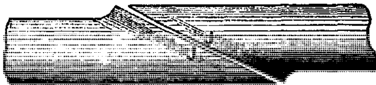
Fig. 83—Showing how the Bars come together.
