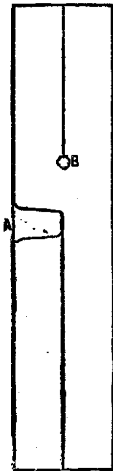
Forging a Dash Foot by "J. C. H." Fig. 197—Showing how the Iron is Fullered, Punched and Split.
