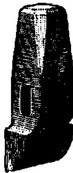
Fig. 6—Large Siding-Down Tool. Made of 1 1/2 square Steel.
