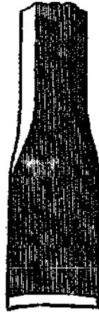
Fig. 48—Improperly Ground Chisel.
