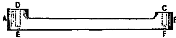
Fig. 38—A Tool designed by "L. G." for making Rivets.
