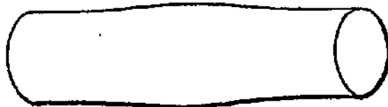
Fig. 93—The Stem prepared to receive the Collar.
