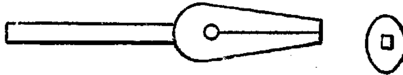
Fig. 251—Side and End Views of the other End after Drawing, Punching and Cutting.
