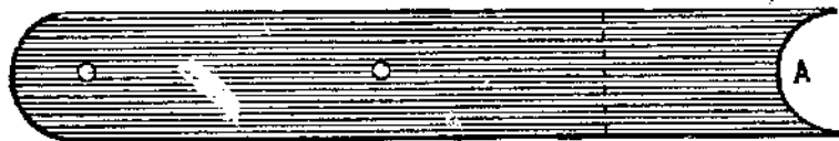
How to Put New Steel Points on Old Plows. Fig. 346—Showing how the First Piece of Steel is Prepared.
