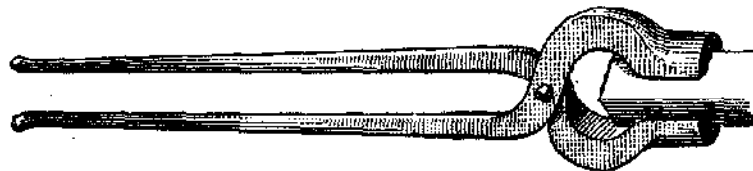
FIG. 98.—TONGS WITH SQUARE, HOLLOW BITS.
