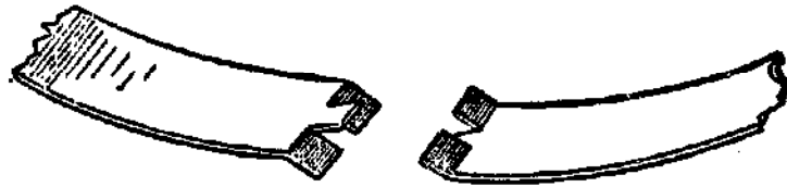
Fig. 98—Welding Springs as Done by a “Jersey Blacksmith.”
