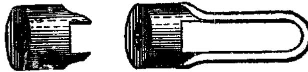
Fig. 147—Showing the Finished Buckle and Collar.
