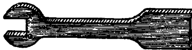
Fig. 60—Shows Faulty Method of Forging Jaws.
