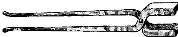
FIG. 99.—FLAT TONGS FOR HOLDING LARGE PIECES.
