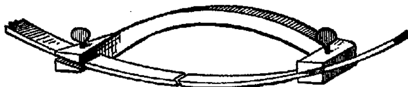
Fig. 73—"D. P.'s" Device for Holding Together Tire Ends While Welding.
