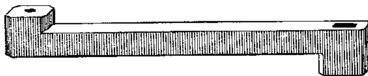
FIG. 68.—SHOWING THE PIECE AFTER WELDING, SHAPING AND PUNCHING.
