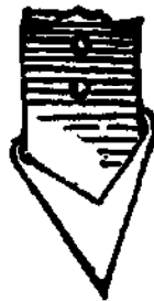
Fig. 389—The Point Adjusted Ready for Welding.
