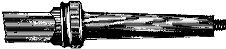
Fig. 167—Well-Rounded Curve Between Arm and Shoulder.
