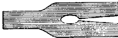
FIG. 181.—SHOWING A FAULTY METHOD OF SPLITTING OUT CROTCHES.
