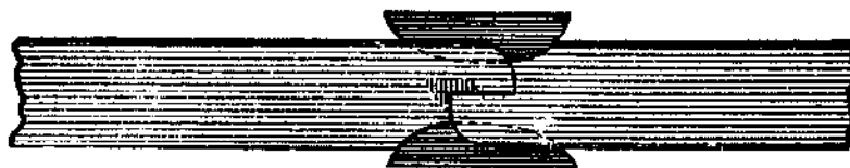
Fig. 95—Welding a Buggy Spring, as done by John Zeck.
