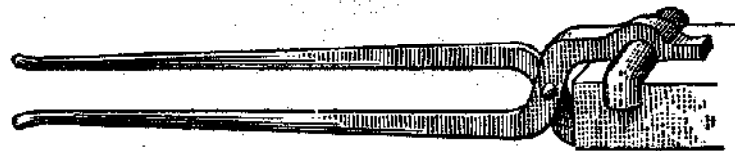
FIG. 95.—SHOWING HOW THE TONGS AND BOX PIECES ARE USED.
