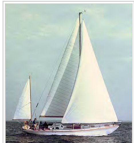
Yawl with triangular jib and main and mizzen sails.
