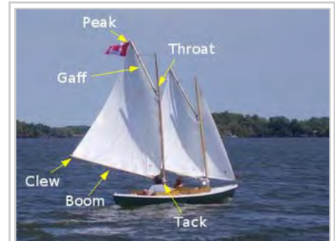
The corners of a quadrilateral fore-and-aft sail.
