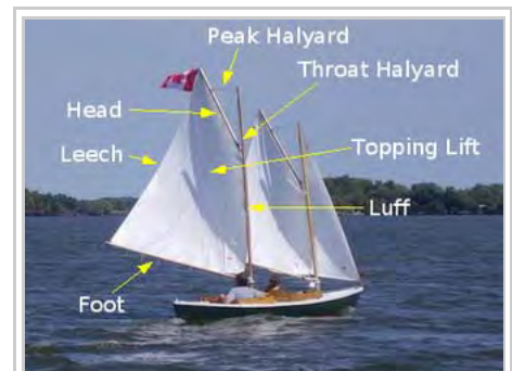
The edges of a quadrilateral fore-and-aft sail.
