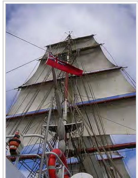
Main-mast of a square-rigged brig.
