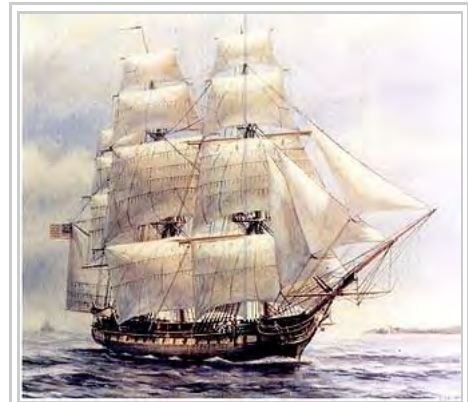
USS Chesapeake , a 1799 United States frigate had triangular jibs and quadrilateral square sails and gaff-rigged sail.
