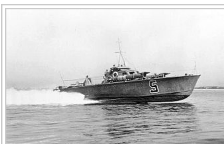
Royal Navy World War II MTB planing at speed on calm water showing its Hard chine hull - note how most of the forepart of the boat is out of the water
