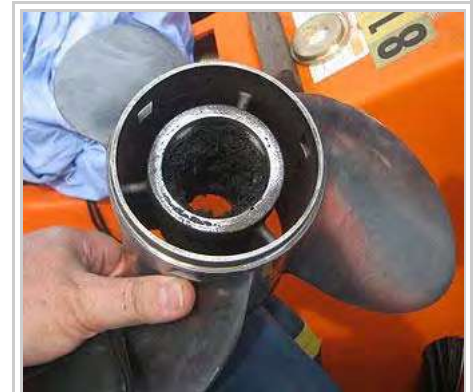
A failed rubber bushing in an outboard's propeller
