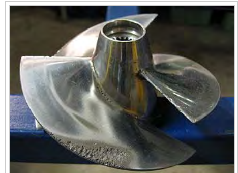
Cavitation damage evident on the propeller of a personal watercraft.
