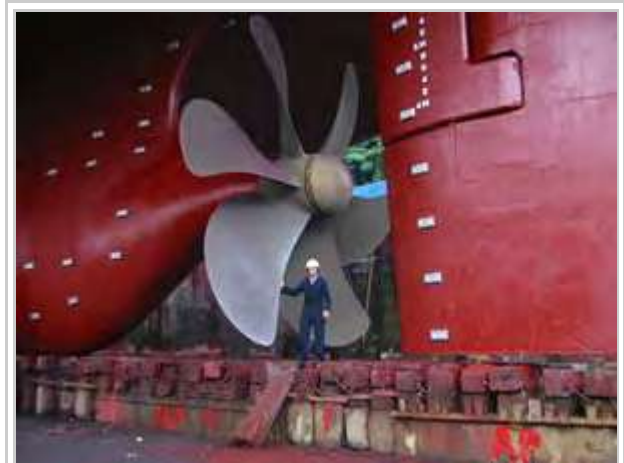
Propeller on a modern mid-sized merchant vessel. The propeller rotates clockwise to propel the ship forward when viewed from astern (right of picture); the person in the picture has his hand on the blade's trailing edge
