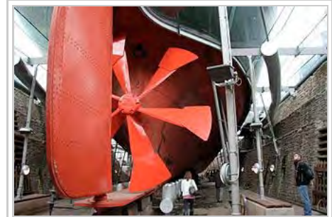
A replica of SS Great Britain 's first propeller was recreated for the museum ship. It was replaced with a four-bladed model in 1845. The SS Great Britain was initially designed to have paddles but was substituted after screw propellers were proven to be more effective and efficient.
