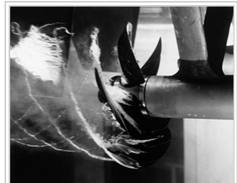
Cavitating propeller in water tunnel experiment
