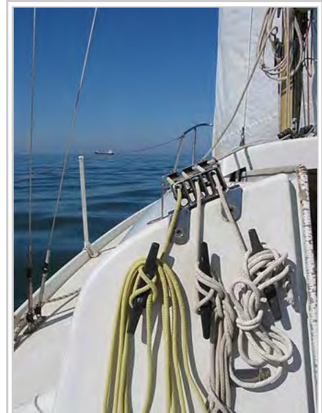
Standing rigging (on the left) and running rigging (on the right), on a sailing boat.
