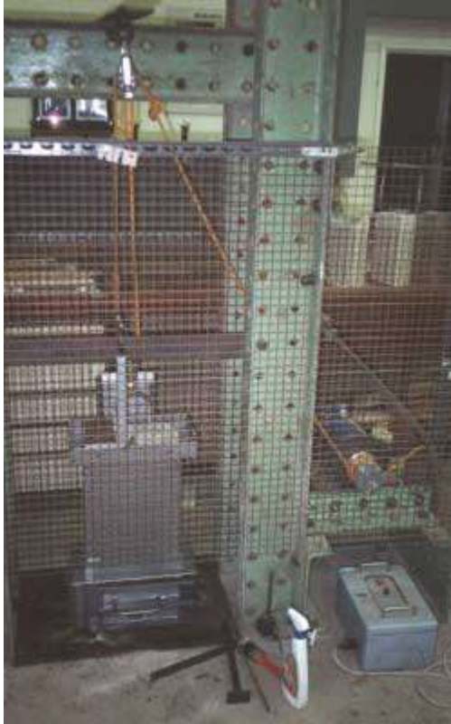
Original test rig (cement impactor)
