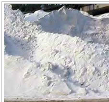
Quartz sand (silica) as main raw material for commercial glass production
