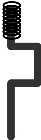
Figure 2: using bent steel rod to rotate drill.
