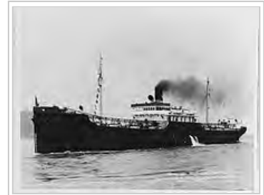
The American concrete oil tanker Palo Alto , originally meant for merchant service in the first World War, but completed in 1919. (Naval History and Heritage Command - Photo NH 799)
