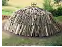
Layer of beech wood around the heart
