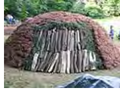
Pile with various layers (wood, spruce brushwood (Fichtenreisig), grass sods)
