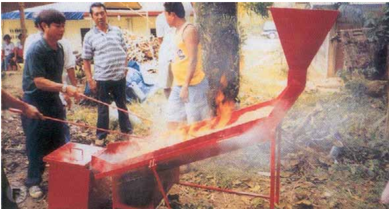
f. The metal plate carbonizer is a simple low-cost machine capable of carbonizing not only sawdust and rice hull but also coconut coir dust and other carbonaceous fine materials.
