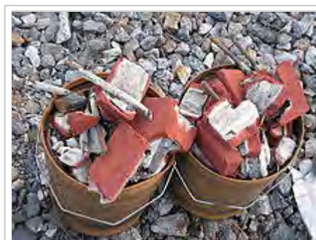
Residues of ceramic molds for thermite welding like these, left by railway workers, can be found along tracks
