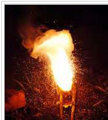
A thermite reaction using iron(III) oxide. The sparks flying outwards are globules of molten iron trailing smoke in their wake.
