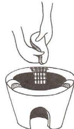
Fig. 4.24 Attaching the pot-rests
