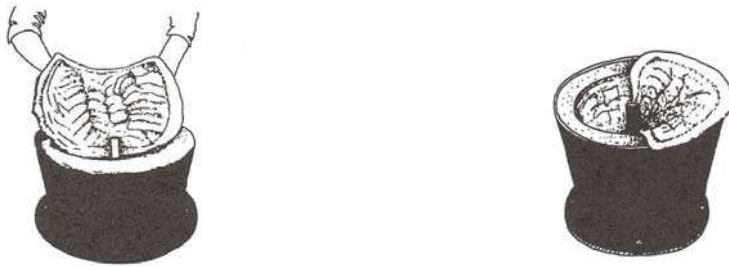
Fig. 4.5 Putting the slabs in the mould and pushing the slabs against the inside walls
