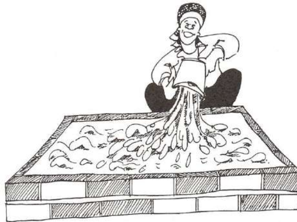
Fig. 3.2 Pit soaking clay
