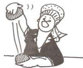
Fig. 4.3 Cutting a block of clay into half and slamming the top half onto the bottom half (wedging)
