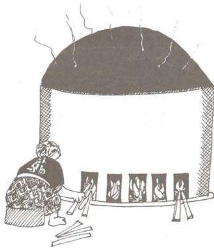
Fig. 5.2 A "Better Bonfire" kiln developed by Intermediate Technology
