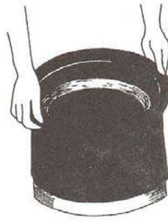
Fig. 4.14 Turning out the liner
