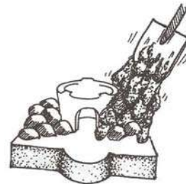
Fig. 7.5 Putting stones and soil around the liner
