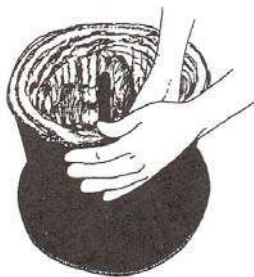
Fig. 4.6 Compacting the seams
