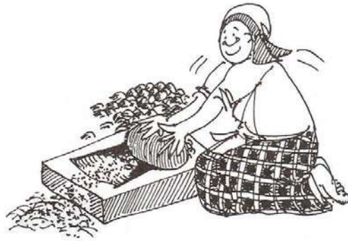
Fig. 3.1 Dry grinding clay
