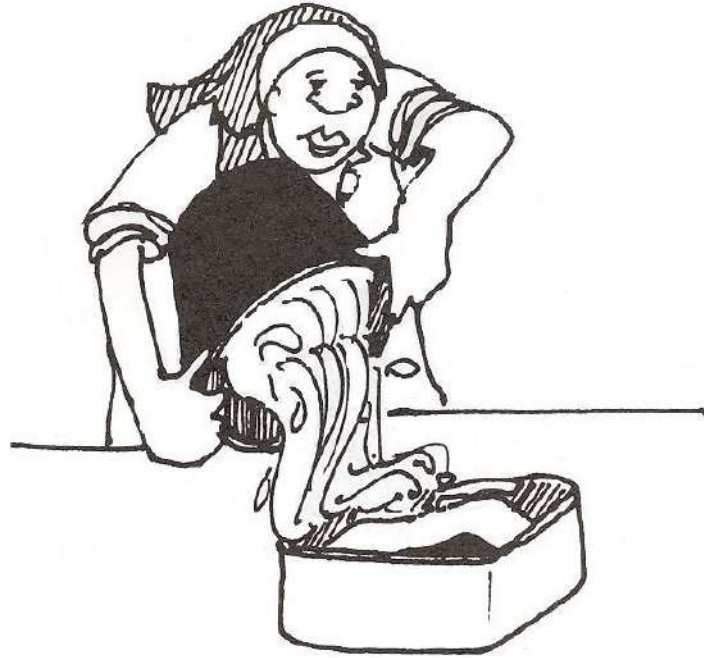
Fig. A1.4 Making a pot-rest mould
