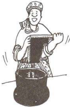
Fig. 4.11 The mould body in the liner
