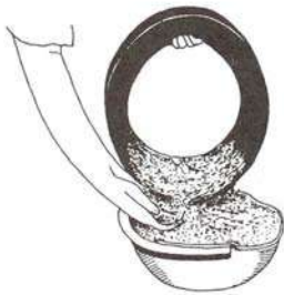
Sprinkling the inside of the mould with ash
