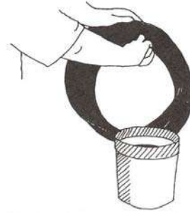
Wiping the inside of the mould
