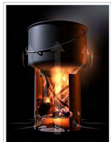
Heat convection in a hobo stove (schematic)
