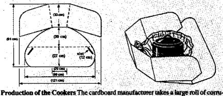
Production of the Cookers The cardboard manufacturer takes a large roll of corrugated cardboard, laminates aluminium foil on one side, and sprays a waterproofing lacquer on the other side. This is then die-cut to form the cooker, complete with the folds and slots. Then they are bundled into loss of 25 (which is about as large as
