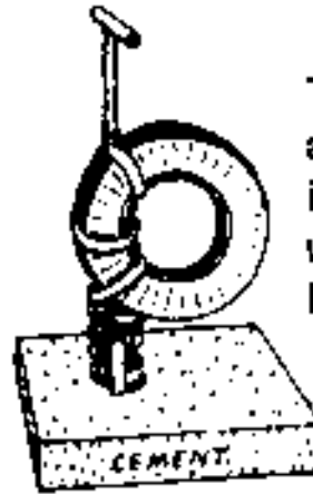
The old design, with the tire suspended by inner-tubes, kept breaking.
