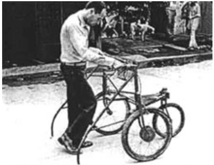
Victor found no walker that could keep him from falling - until he created this five point system. The rear pipes add stability and act as extra brakes, along with the hand brakes.
