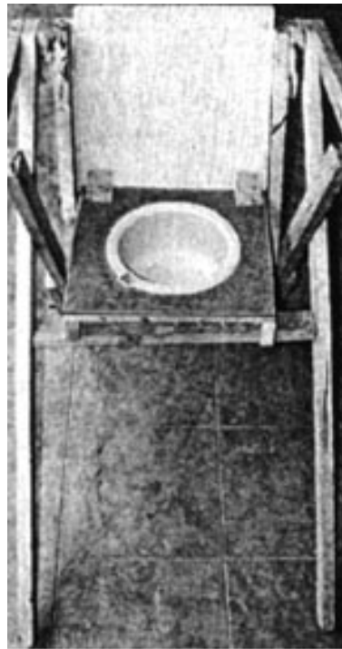
Toilet seat of the walker with the lid lifted out of the way.
