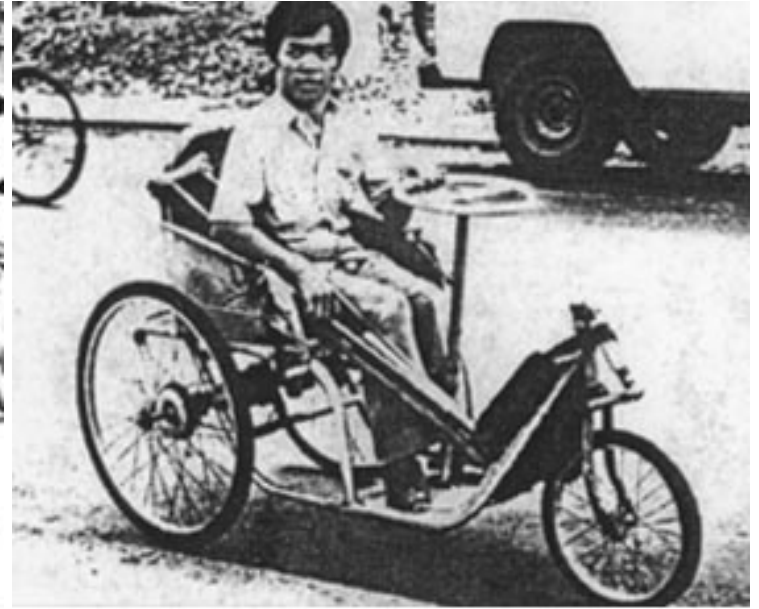
Vietnam. Designed in France. Steering column pumps back and forth to give dual rear-wheel drive.
