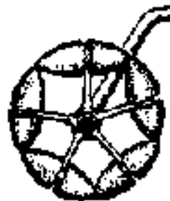
Ralfs "Ezekiel wheel." The small rollers roll sideways. The main wheel rolls forward. This gives a multi-directional caster effect, without swiveling.
