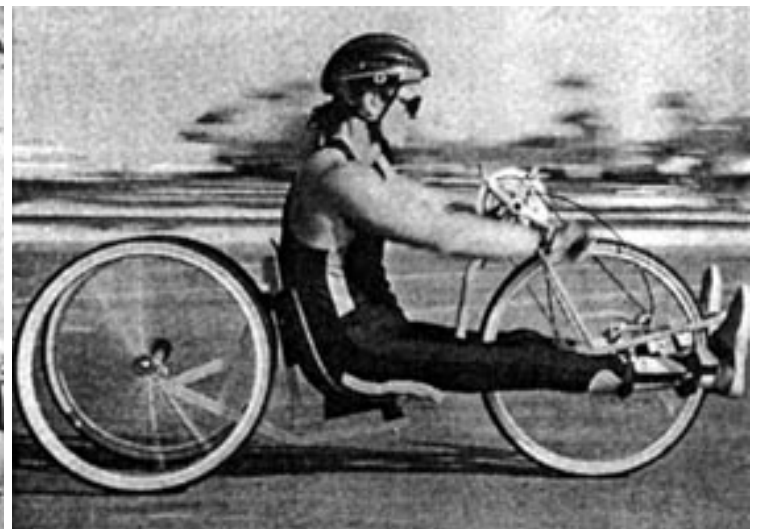
Racing trike. Sold commercially in USA. Front-wheel drive. Rider's forward position increases traction.
