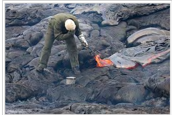
A volcanologist sampling lava using a rock hammer and a bucket of water
