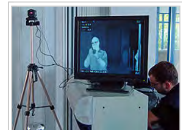
Thermal imaging camera and screen, photographed in an airport terminal in Greece during the 2009 flu pandemic. Thermal imaging can detect elevated body temperature, one of the signs of swine flu.
