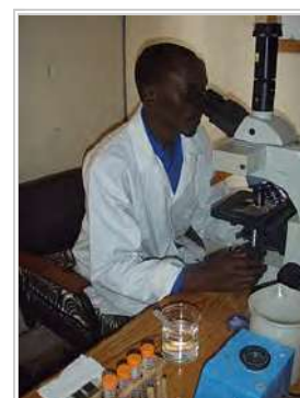
Analysing for helminth eggs in samples of feces from a dry toilet in Kenya
