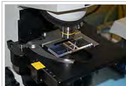
A Neubauer slide held in place on a microscope stand by a slide clamp on a cross-table.
