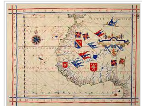
A pre-Mercator nautical chart of 1571, from Portuguese cartographer Fernão Vaz Dourado (c. 1520–c. 1580). It belongs to the so-called plane chart model, where observed latitudes and magnetic directions are plotted directly into the plane, with a constant scale, as if the Earth were a plane (Portuguese National Archives of Torre do Tombo, Lisbon).
