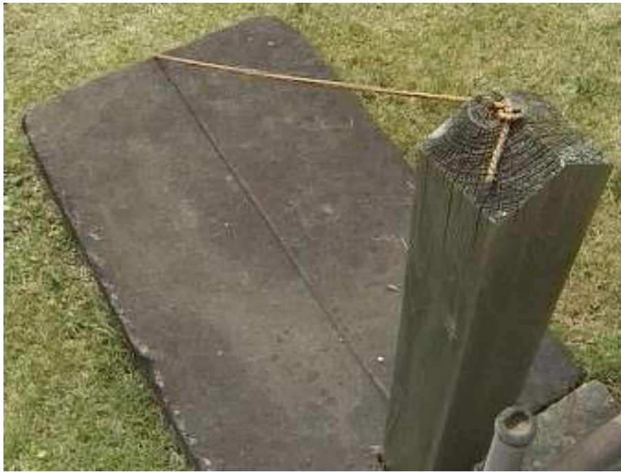
Photo of the "sun clock" taken at noon; note the shadow of the string roughly coincides with the linear marking on the stone.
