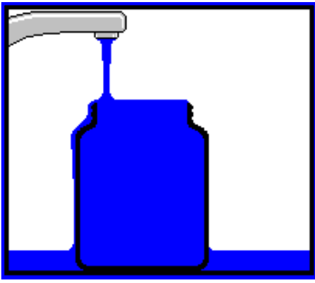
Fig. 7 Constant overflow cleans the surface
