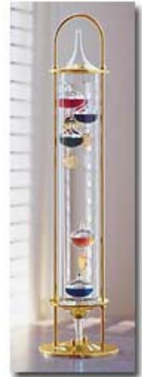
Galileo Thermometer Photo courtesy: Wind & Weather
