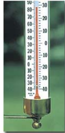
Bulb Thermometer Note reservoir at bottom. Photo courtesy: Wind & Weather
