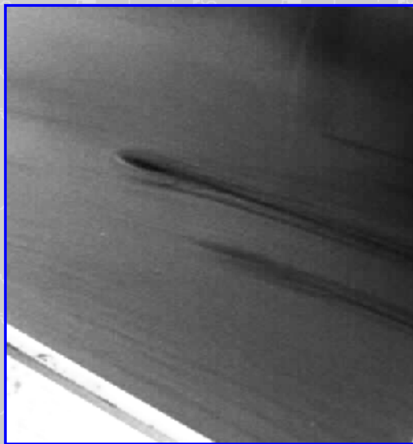
Fig. 2 Not the surface of Jupiter, but the slot made in the flowing CO2 fog by a single "air-thread." The emitter is a human hair 1/4" long, held two feet away. Two other marks are also visible, no doubt made by tiny bits of lint on the cliplead which held the hair. The part of the stripe visible here is about 4 inches in length.
