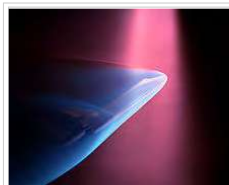
During a NASA wind tunnel test, a model of the Space Shuttle is targeted by a beam of electrons, simulating the effect of ionizing gases during re-entry. [157]
