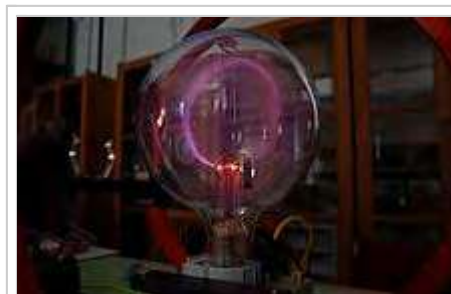
A beam of electrons deflected in a circle by a magnetic field [27]
