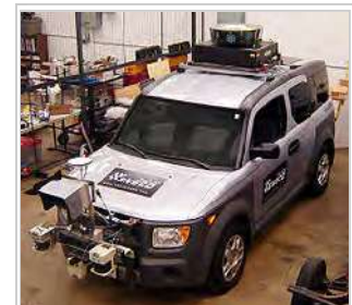
Radar, GPS, lidar, ... are all combined to provide proper navigation and obstacle avoidance (vehicle developed for 2007 DARPA Urban Challenge)
