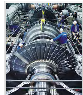
Design of a turbine requires collaboration of engineers from many fields, as the system involves mechanical, electro-magnetic and chemical processes. The blades, rotor and stator as well as the steam cycle all need to be carefully designed and optimized.
