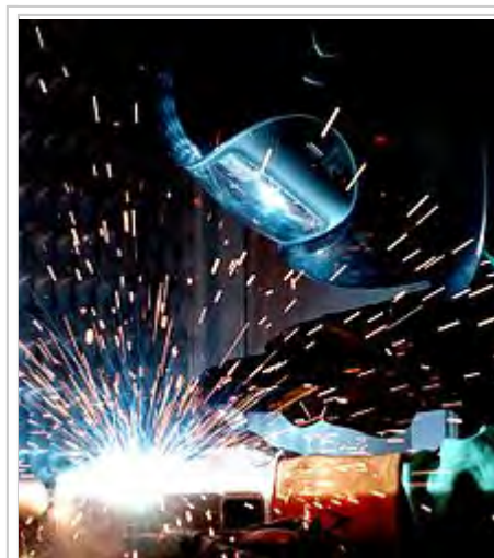
Arc welders need to protect themselves from welding sparks, which are heated metal particles that fly off the welding surface.
