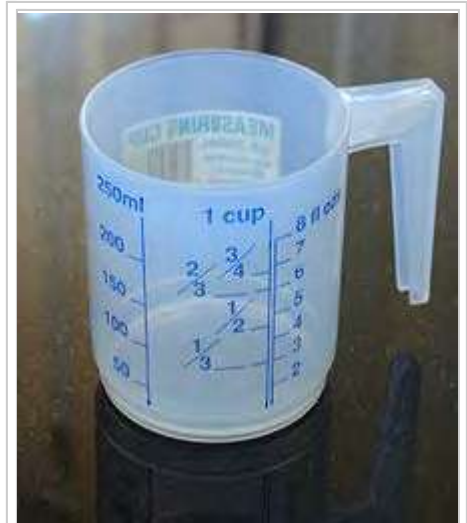
A measuring cup can be used to measure volumes of liquids. This cup measures volume in units of cups, fluid ounces, and millilitres.
