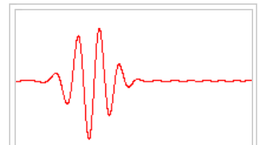
A propagating wave packet; in general, the envelope of the wave packet moves at a different speed than the constituent waves. [28]
