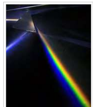
Light beam exhibiting reflection, refraction, transmission and dispersion when encountering a prism
