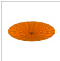
A two-dimensional standing wave on a disk; this is the fundamental mode.
