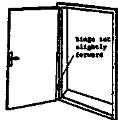
9 Correct fixing of door, with door slightly open
