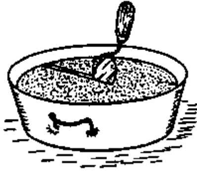
Fig. 2: MAKE A CUT WITH THE TROWEL
