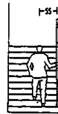
If stairs are wide and straight, distance of walk line from handrail is 550 mm (22 in)
