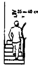
If stairs are narrow or curved, distance of walk line from outer edge is 350-400 mm (14-16 in)
