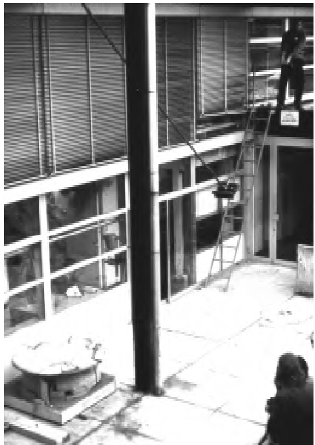
3-3 Simulation of seismic shocks (Minke 2000)
