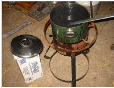
(2) DIY machineable wax is 1 part polyethylene to 4 parts wax.
