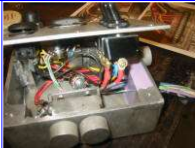
(5) RTV seals the helm control box from water and provides a strain relief for the wires.
