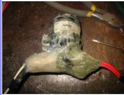
(9) A 100 amp solenoid relay potted in epoxy. A plastic bag and clay were used make molds for the epoxy.
