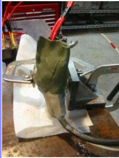
(8) Modeling clay used to make a mold for epoxy around wire terminals on a relay.
