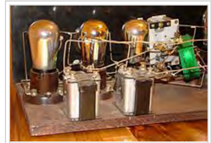
This 1920s TRF radio manufactured by Signal was constructed on a wooden breadboard.
