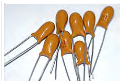
Solid electrolyte, resin-dipped 10 \mu F 35 V tantalum capacitors. The + sign indicates the positive lead.
