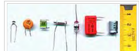
Capacitor materials. From left: multilayer ceramic, ceramic disc, multilayer polyester film, tubular ceramic, polystyrene, metalized polyester film, aluminum electrolytic. Major scale divisions are in centimetres.
