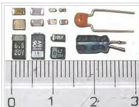
Capacitor packages: SMD ceramic at top left; SMD tantalum at bottom left; through-hole tantalum at top right; through-hole electrolytic at bottom right. Major scale divisions are cm.
