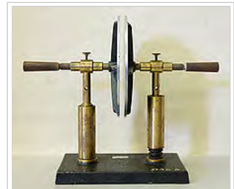
A simple demonstration capacitor made of two parallel metal plates, using an air gap as the dielectric.
