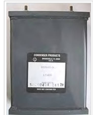
This mylar-film, oil-filled capacitor has very low inductance and low resistance, to provide the high-power (70 megawatt) and high speed (1.2 microsecond) discharge needed to operate a dye laser.
