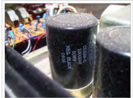
A 10,000 microfarad capacitor in an amplifier power supply
