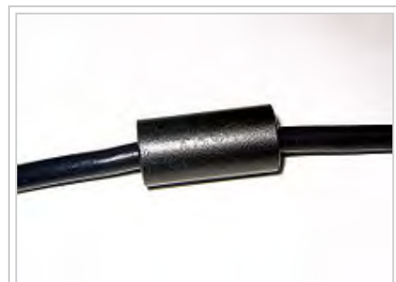
A ferrite "bead" choke, consisting of an encircling ferrite cylinder,
