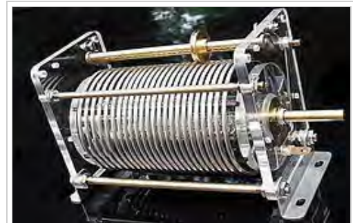
A "roller coil", an adjustable air-core RF inductor used in the tuned circuits of radio transmitters. One of the contacts to the coil is made by the small grooved wheel, which rides on the wire. Turning the shaft rotates the coil, moving the contact wheel up or down the coil, allowing more or fewer turns of the coil into the circuit, to change the inductance.
