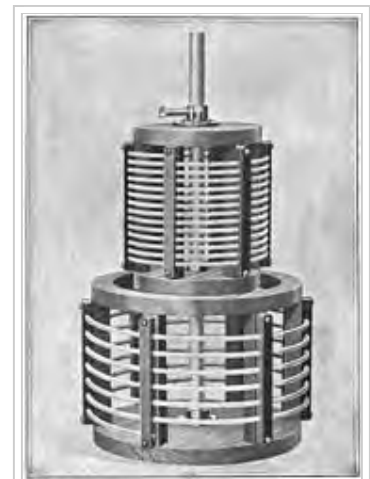
Resonant oscillation transformer from a spark gap transmitter. Coupling can be adjusted by moving the top coil on the support rod. Shows high Q construction with spaced turns of large diameter tubing.
