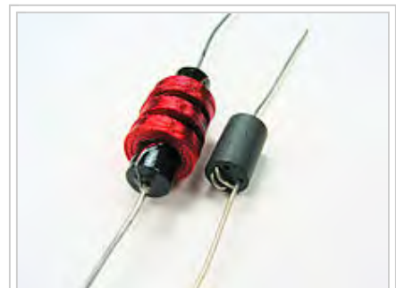
An MF or HF radio choke for tenths of an ampere, and a ferrite bead VHF choke for several amperes.
