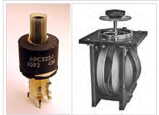
(left) Inductor with a threaded ferrite slug (visible at top) that can be turned to move it into or out of the coil. 4.2 cm high. (right) A variometer used in radio receivers in the 1920s
