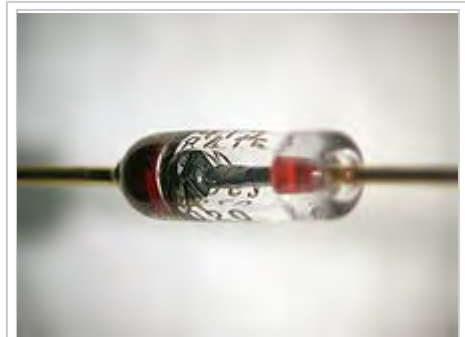
Closeup of a diode, showing the square-shaped semiconductor crystal ( black object on left ).
