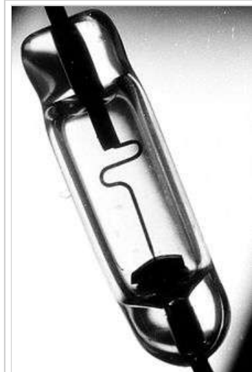
Closeup of a diode, showing the square-shaped semiconductor crystal ( black object on left ).
