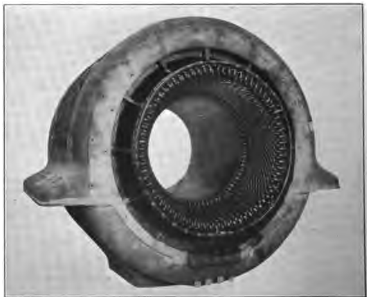
FIG. 237. — Stationary armature of figure 236 for high-speed alternator.
