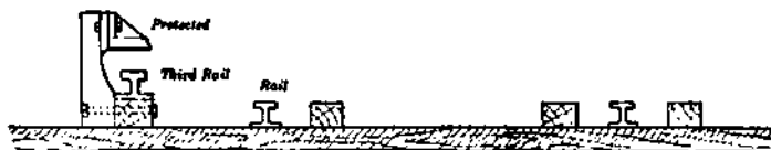
FIG. 352. — Third rail protected by a wooden shield.
