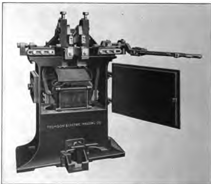
FIG. 345. — Thomson automatic electric welder with step-down transformer in case beneath. The secondary winding is but a single turn. The regulator switch is on the outside of case at left. On top is a stationary head (left) and a movable head (right) to hold the pieces to be welded. The compression lever with switch handle are at the extreme right.
