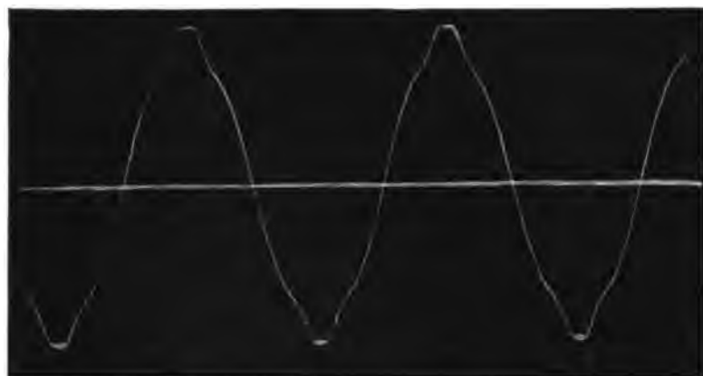
FIG. 248. — Actual voltage curve at no load. 150 kv-a. and 60 cycles.
