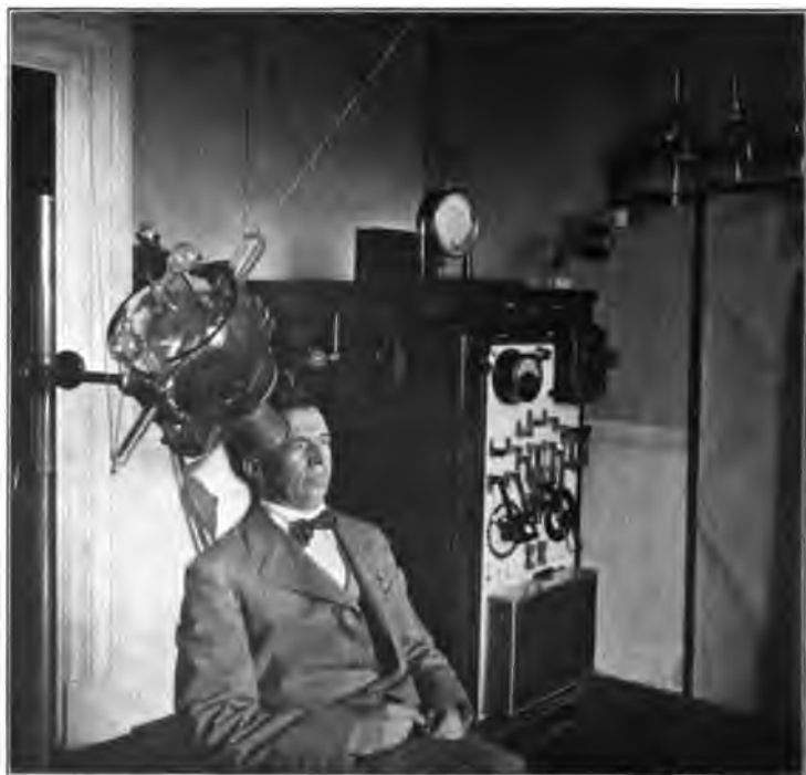
FIG. 431. — Radiographic apparatus arranged for use in a dental hospital. (Photographic film inside patient's mouth.)
