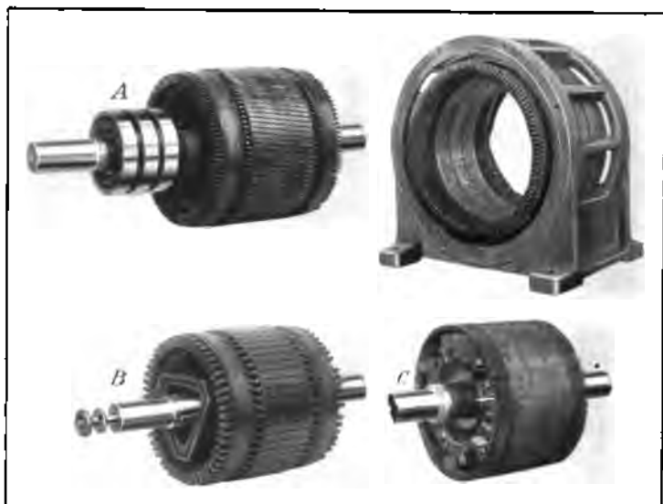
FIG. 271. — Various types of rotors for same stator. A , wound rotor with slip rings; B , wound rotor with internal resistance controlled by lever from end of shaft; and C , squirrel-cage rotor with ventilating vanes.
