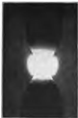
FIG. 321. — Open arc produced by alternating current.
