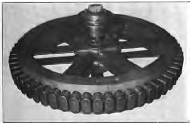
FIG. 238. — Revolving field with 60 poles used with reciprocating steam engines and water wheels.
