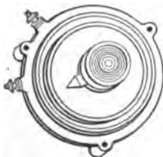
FIG. 150. — View of field rheostat with its connections.
