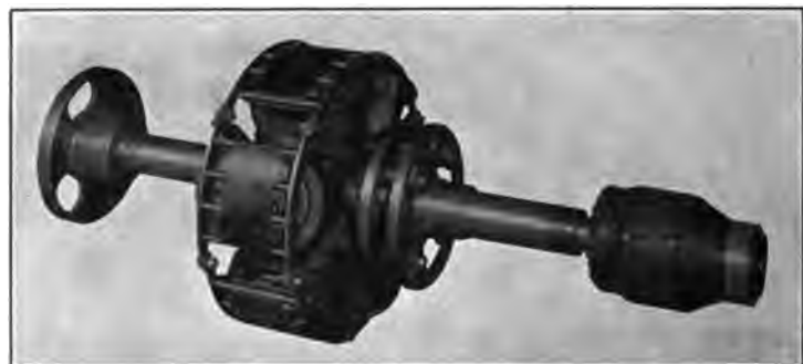
FIG. 241 a. — Shaft with rotating field and exciter armature. Note grids across pole faces.
