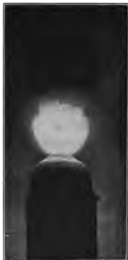
FIG. 320. — Electric arc produced by direct current.
