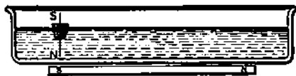
FIG. 41. — Experiment to illustrate the movement of a free magnetic pole when near a bar magnet.
