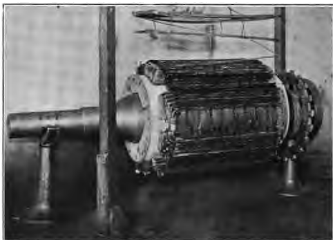
FIG. 236. — Cylindrical form of partly wound revolving field used with steam turbines. It has 4 poles.
