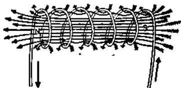
FIG. 49. — Loose solenoid with its lines of force.
